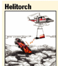
A device carried by helicopter for dropping ignited lumps of gelled gasoline. Setting oil ablaze is one way Shell says it can clean up a spill in ice-choked seas.
